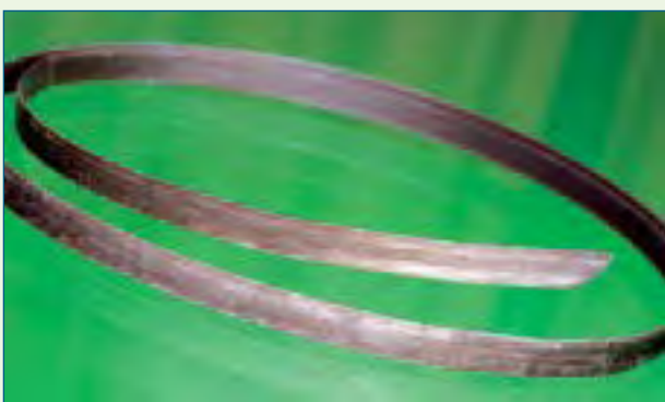
figure co.2 The magnesium oxide coating needs to be removed when performing experiments with magnesium ribbon.
